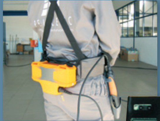
1,1 kg (2.2 lbs) portable battery pack with autonomous operation display
